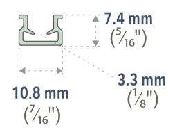
Accommodates 1/8", 3/16" and 1/4" panels Remove one lip for a 3/16" panel Remove both lips for a 1/4" panel
